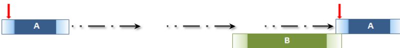
Figure 8: Temporal entity A starts before or with the end of temporal entity B. Here A is shorter than B
